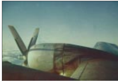
2) a side view showing oil streaks along the cowling
